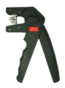
CC\$12 Cable Stripper is suitable for stripping wire sizes from 0.75-16mm<sup>2</sup>.
